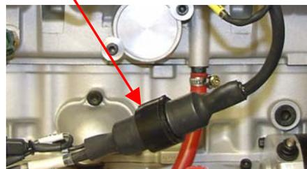
If you are using a standard Suzuki injector harness then it may have a fuel pump output as pictured below, if so then you can plug this directly into a standard fuel pump, or if you are using an aftermarket pump such as our own FP1 (as pictured in the previous pages) then you will require an extension lead.
