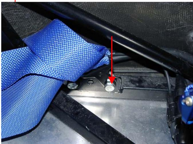
The chassis ground should be connected to either the battery negative or a good chassis ground as show. PLEASE ENSURE VERY CLEAN SURFACES.
