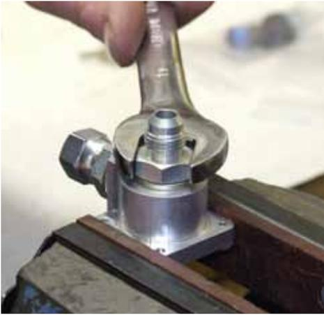
Tighten connections on fuel regulator mount.
