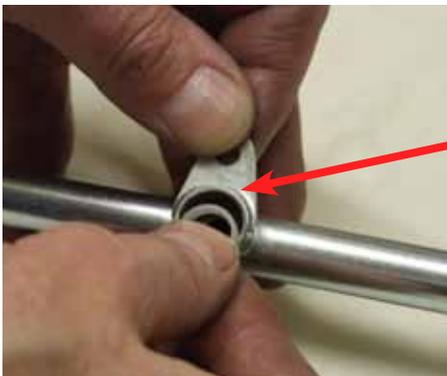
Insert the injectors spacers into the fuel rail
