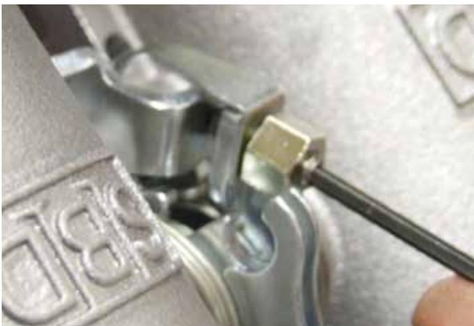
When finally locking up use an allen key at the same time as the spanner to ensure you do not accidentally move the adjusters. Finally re-check the whole set-up.
