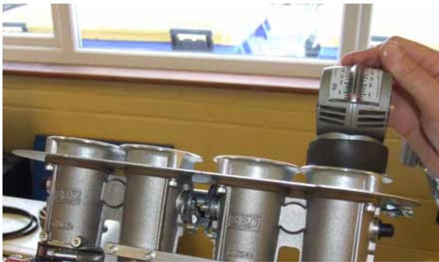
6. You now need to adjust the throttle position sensor to read the correct idle voltage. If you fail to set the throttle pot to the correct voltage, the engine is likely to not respond well when the throttle is opened (picture 9)
