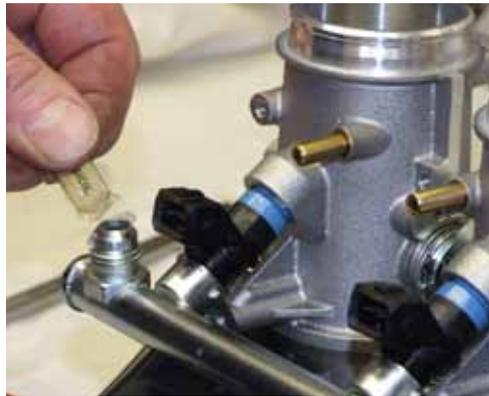
Lubricate the regulator o-ring with a small amount of silicon (provided with the injectors).
