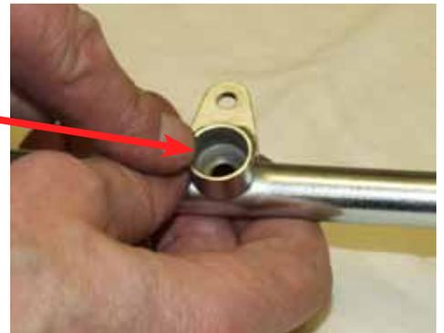
Put silicon on the injector o-rings & insert into the fuel rail.
