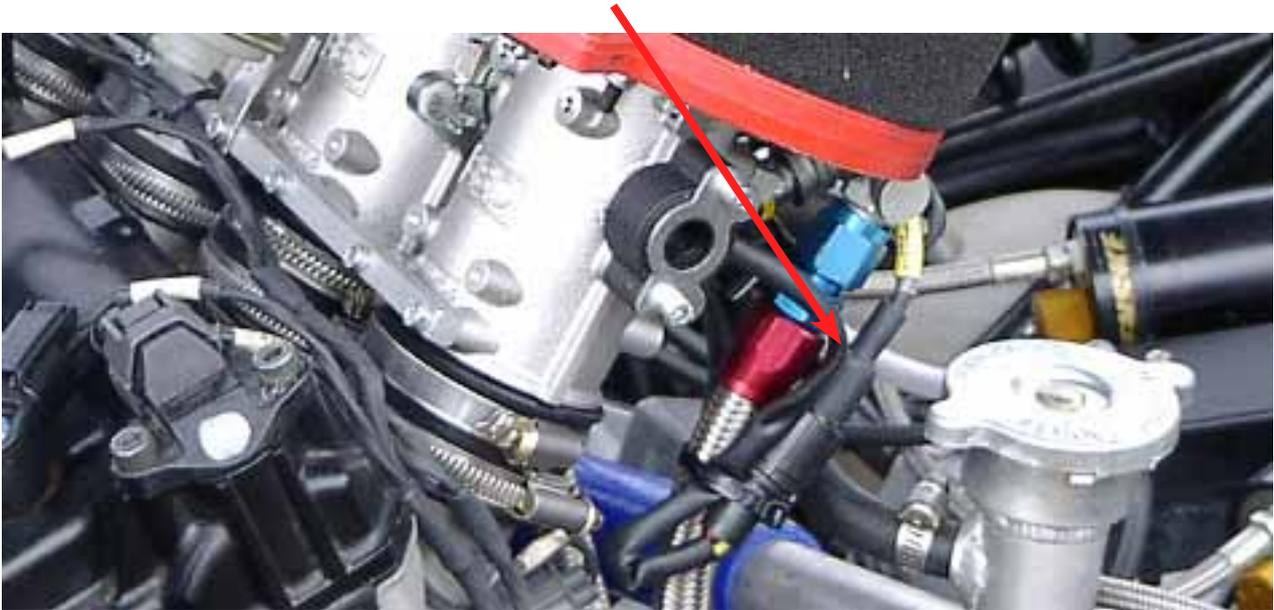
2. With the ignition on & engine NOT running set the voltage to less than the idle voltage, by loosening the 2 screws & twisting the pot. (e.g. 0.3 volts) This is an ideal starting point.
