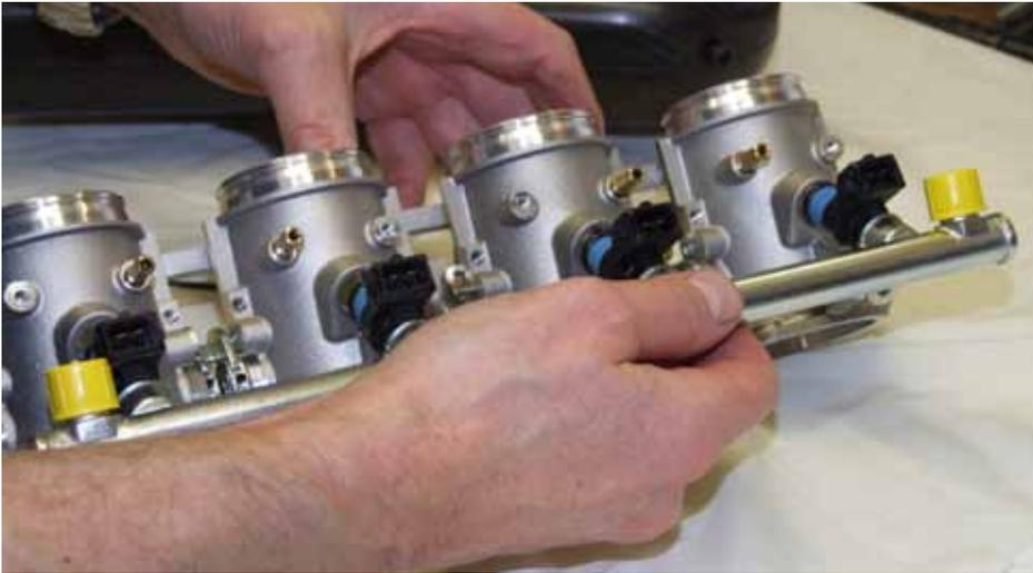
Please note that the brass bleed valves are only used on Turbo & Supercharged applications
