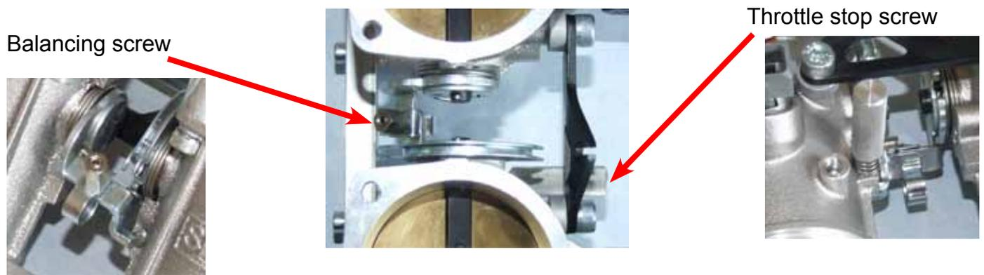
5. Using the throttle stop screw, adjust the butterflies until the kilograms of air per hour are correct for your engine specification (pictures 5-8) see table at the beginning of Set up procedure.
