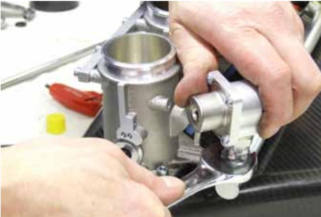
Insert the regulator into the mount & tighten the bolts.
