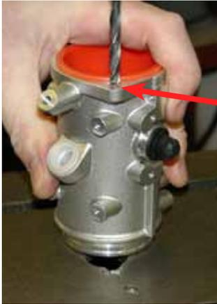
In order to fit the short air horns to your throttle bodies, the holes must be drilled out to 5.50mm. This should be done before fitting the throttle bodies together.
