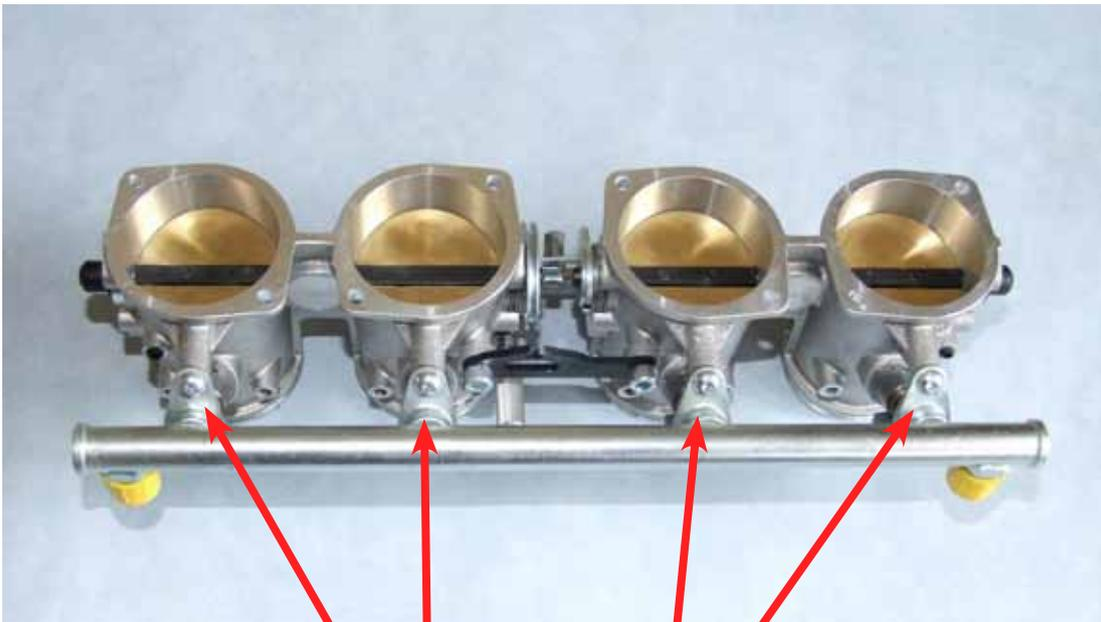
Attach the fuel rail & injectors to the throttle bodies & tighten all the bolts
