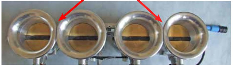
If you are using the short air horns, they will need to be bolted from the throttle body side into the air horns (see below & right), insert all the bolts loosely & once the air horns are all fitted tighten bolts.
