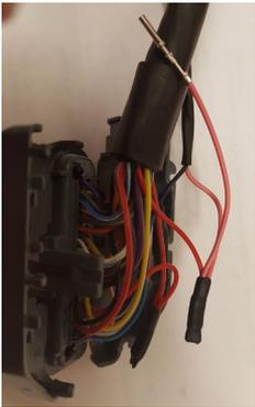
Next slide the short piece of glued heat shrink provided over the three wires so the crimp is completely enclosed along with the ends of the three wires.
