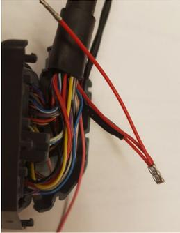
Then group all three wires together, slide the metal crimp over them and then crimp down gently so they are all retained.
