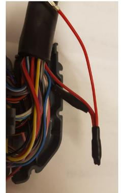
Neatly fold back the wires within the hood making them as tidy as possible to allow you to squeeze the grey hood back together, this part may take a bit of time but the wires will press down neatly.
