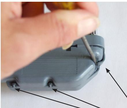
Careful loosen the 3 retaining clips using a small flat-bladed screwdriver to open the connector.
