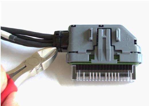
Remove cable tie using side cutters, being very careful not to damage the wires & heat shrink.
